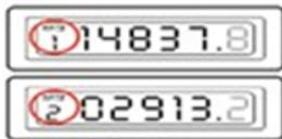
**Two rate meters** - only have one digital display. They will either flash up the different rate readings in a cycle or have a button that you need to press to make the display cycle through the readings for the different rates. The 5 numbers shown left to right are the numbers you need for both readings - ignore the number(s) after the decimal point which may be shown in red.
