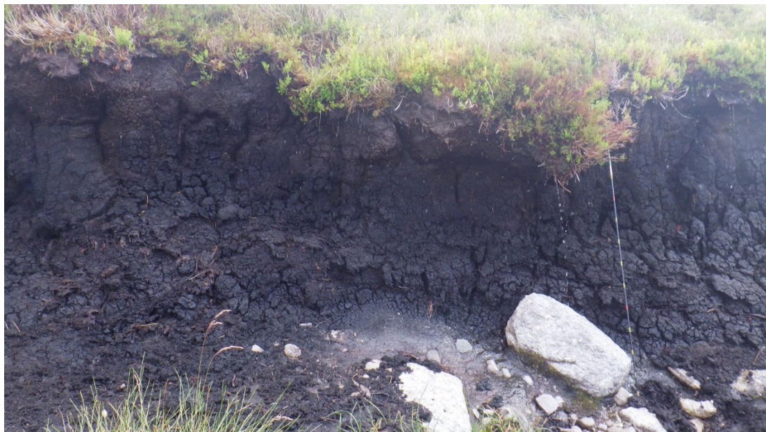
Photograph 10.4.1: Exposed diamicton till and morainic deposits underlying surface peat, NGR NC 6164 1844. Peat in this location is approximately 1.5 m in thickness.
